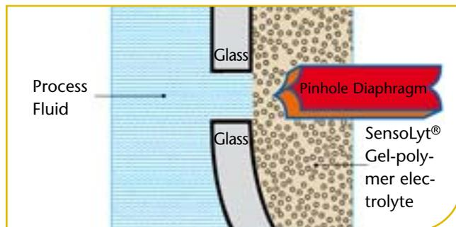
The reliability of pH and ORP measurements are determined to a large extent by the quality of the pH/ORP electrode which commonly is exposed to extreme conditions; particularly in many industrial applications.
